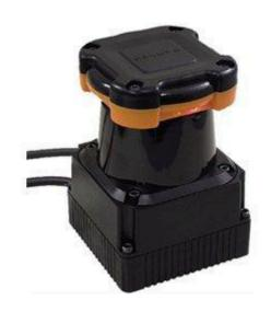
The **Hokuyo UTM-30LX Scanning Laser Rangefinder** is a small, affordable and accurate laser scanner that is perfect for robotic applications. The **UTM-30LX** is able to report ranges from 100mm to 30m (1mm resolution) in a 270° arc (0.25° angular resolution). Its power consumption — 12V 700ma — allows it to be used on battery operated platforms.
