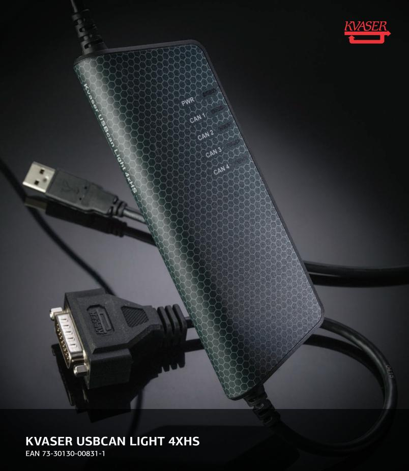
The USBcan Light 4xHS is a compact, reliable and cost-effective means of connecting four high-speed CAN busses to a PC or mobile computer. With galvanic isolation as standard, this USB to quad channel CAN interface has a standard USB connector at one end and four high speed CAN channels in a single 26-pin HD D-SUB CAN connector at the other. The supplied HD26-4xDS9 splitter can be used to connect to four separate 9-pin D-SUB connectors.
