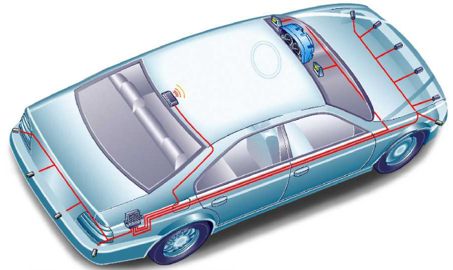
Typical parking aid system configuration (maximum 12 sensors per vehicle)
