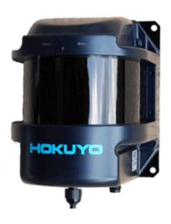
The Hokuyo UXM-30LX-EW Scanning Laser Rangefinder is in many ways Hokuyo's most farsighted scanner. Normal objects can be seen up to 50m away, while those difficult to see "low reflectance" objects (10% reflectivity & above) can be seen from a distance of 30m. Additionally, the multi-echo functionality ensures that low level "noise" caused by adverse weather conditions such as snow, rain, fog and dust, is filtered out.
