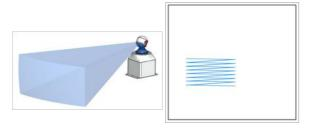
Region Scanning — This mode allows the user to define a rectangular region within the scanner's azimuth and elevation field in which to concentrate the scanning. The Region Scan mode gives the most control over the attention of the scanner with scan rate, number of lines per degree, sample rate and sample averaging parameters available as in other modes. Region Scanning is most useful when a region's extent in azimuth is less than 60°.
