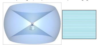
Full Field Scanning — Allows scans to be defined that cover the full 360° azimuth by 70° elevation field of the scanner. Parameters to adjust the azimuth scan rate, the number of lines per degree in elevation, the sample rate and sample averaging are available in this mode. These parameters enable the resolution of the resulting 3D data in both azimuth and elevation to be traded off against acquisition time to best meet the requirements of the application at any point in time.
