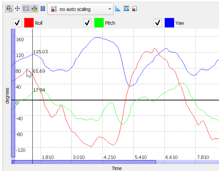
Figure 26: The Show Values button activates the possibility to see the values in the graph
