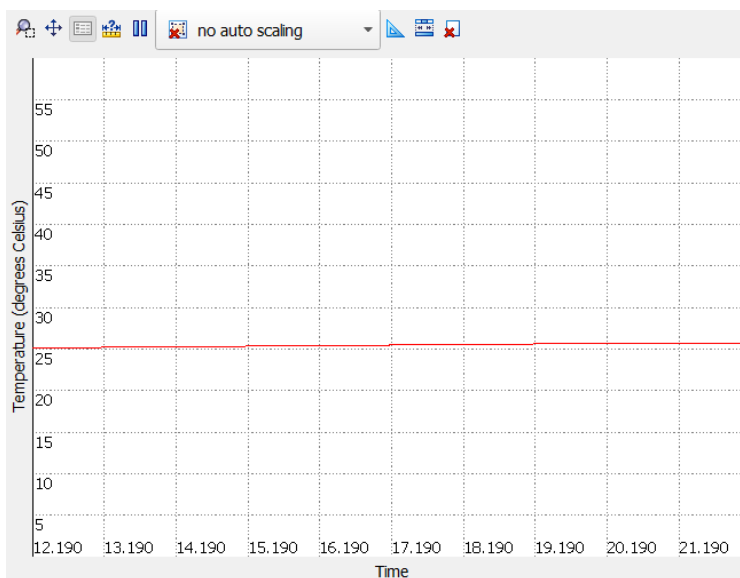
Figure 33: The Temperature view window, showing that the MTi is warming up directly after powering it.
