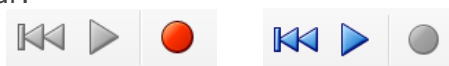
Figure 43: The Playback and recording bar when an MTi is attached (left) and when a file is loaded in MT Manager (right)
